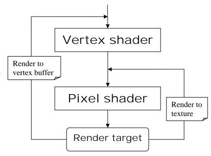
actual geometry. R2VB solves the problem by looping the data back even further, all the way to the vertex shader. This simple diagram demonstrates the difference.
